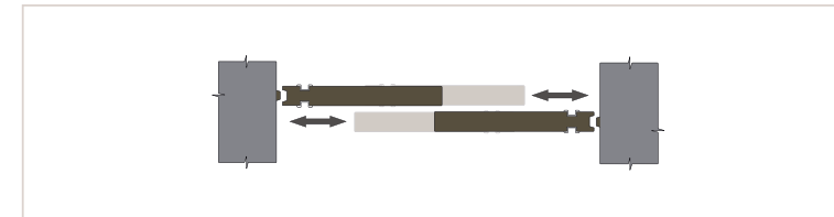
2 ante scorrevoli parallele, binario a 2 vie / Double parallel sliding door, 2 ways rail
